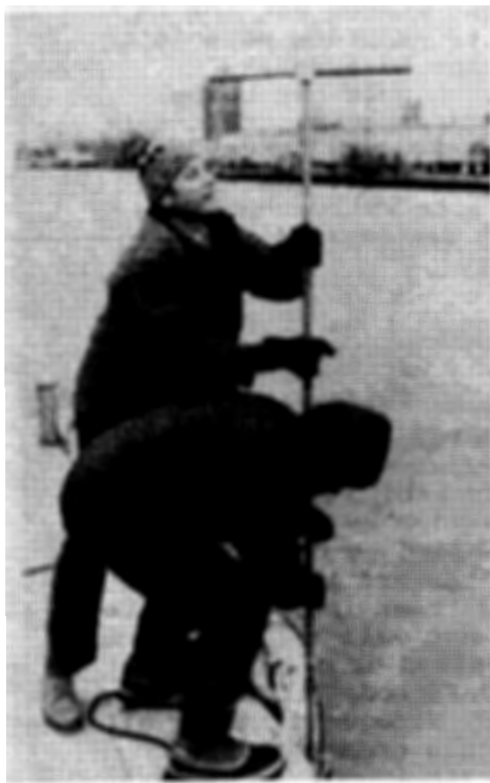
Taking sediment core samples near Slip 3 in Waukegan Harbor to use in PCB toxicity study (Project #010).
