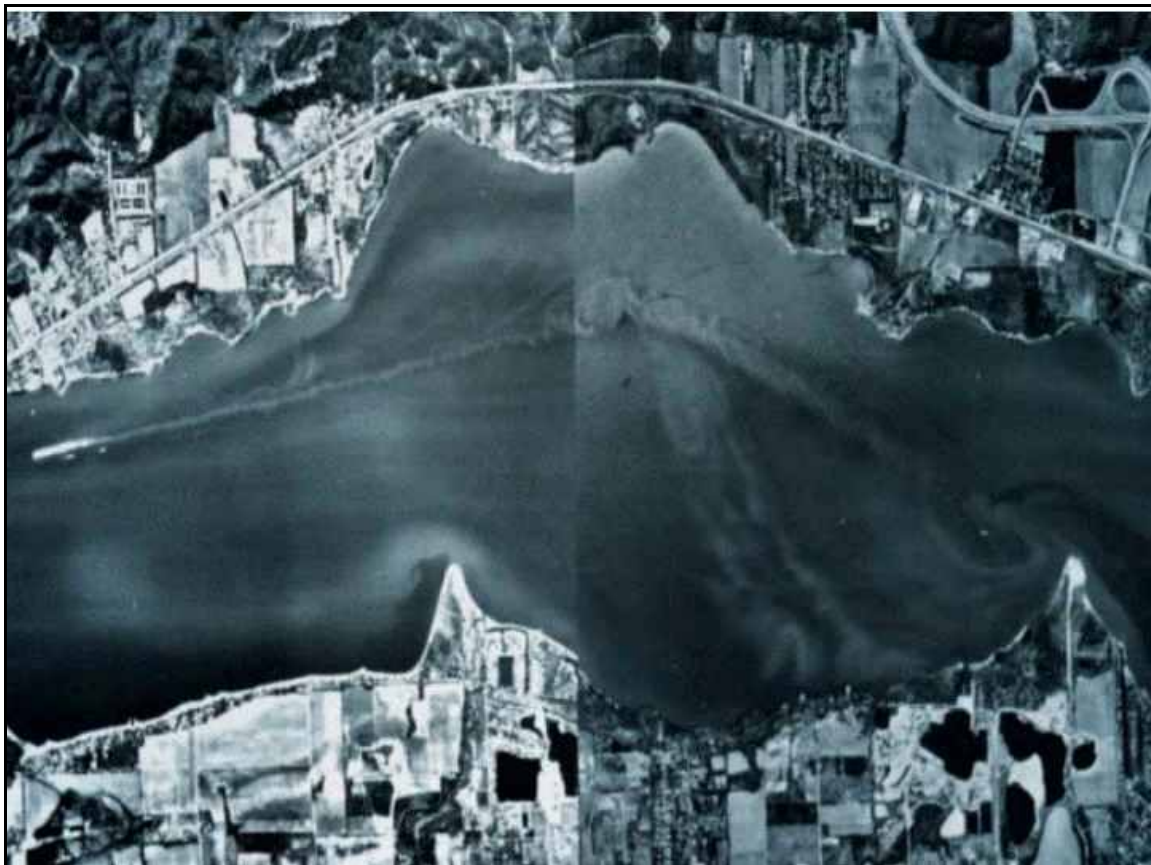
Figure 2. Fine grained sediment is easily resuspended, especially in shallow water. In this picture a suspended sediment plume several miles long is visible behind a barge tow in Upper Peoria Lake. Plumes of varying lengths are also generated by fish and recreational craft.
