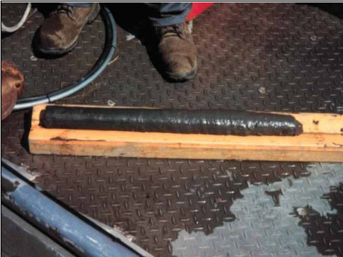
Figure 3. Sediment cores up to nine feet in length show that the sediment is soft but relatively firm. As seen above a fresh core keeps its shape and loses little water. If the sediment can maintain its in place consistency during excavation, it will be much easier to build islands or dewater on shore for other uses.
