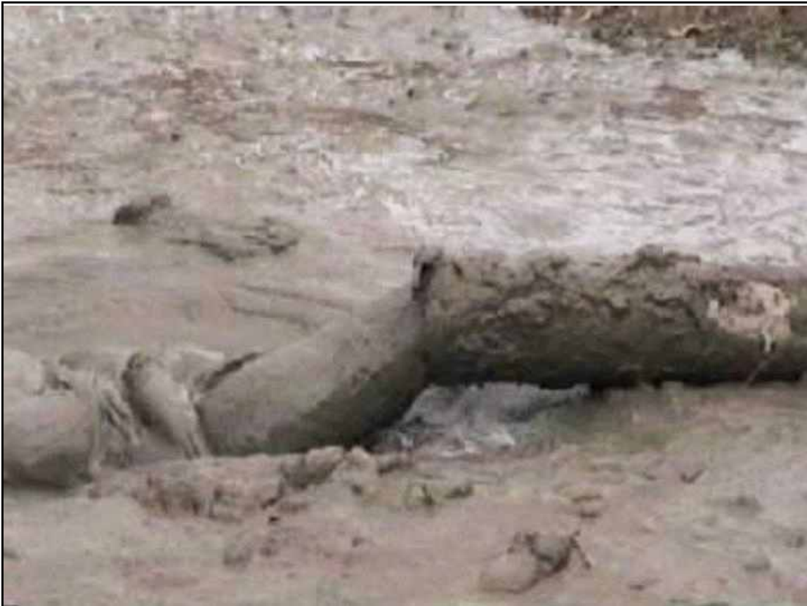
Figure 5. The DRY DREdge (TM) by DRE , Inc. uses a small clamshell bucket and a displacement pump to remove and transport sediment at essentially its in situ moisture content. The discharge above is about the consistency of toothpaste. The current working model has a low capacity compared to conventional machines.
