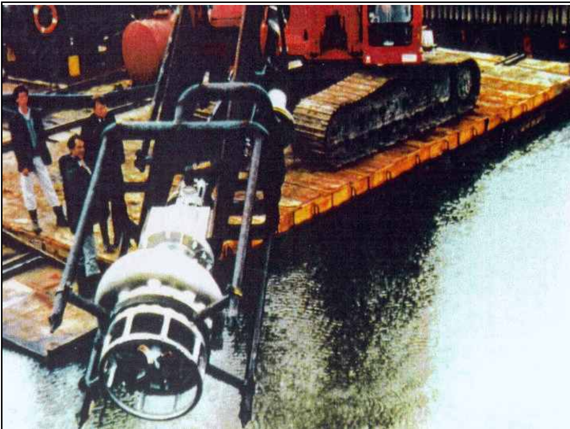
Figure 4. A number of companies make pumps which are capable of handling material with a high solids content. The pumps are available in various sizes and can be mounted on conventional excavator arms or cranes.
