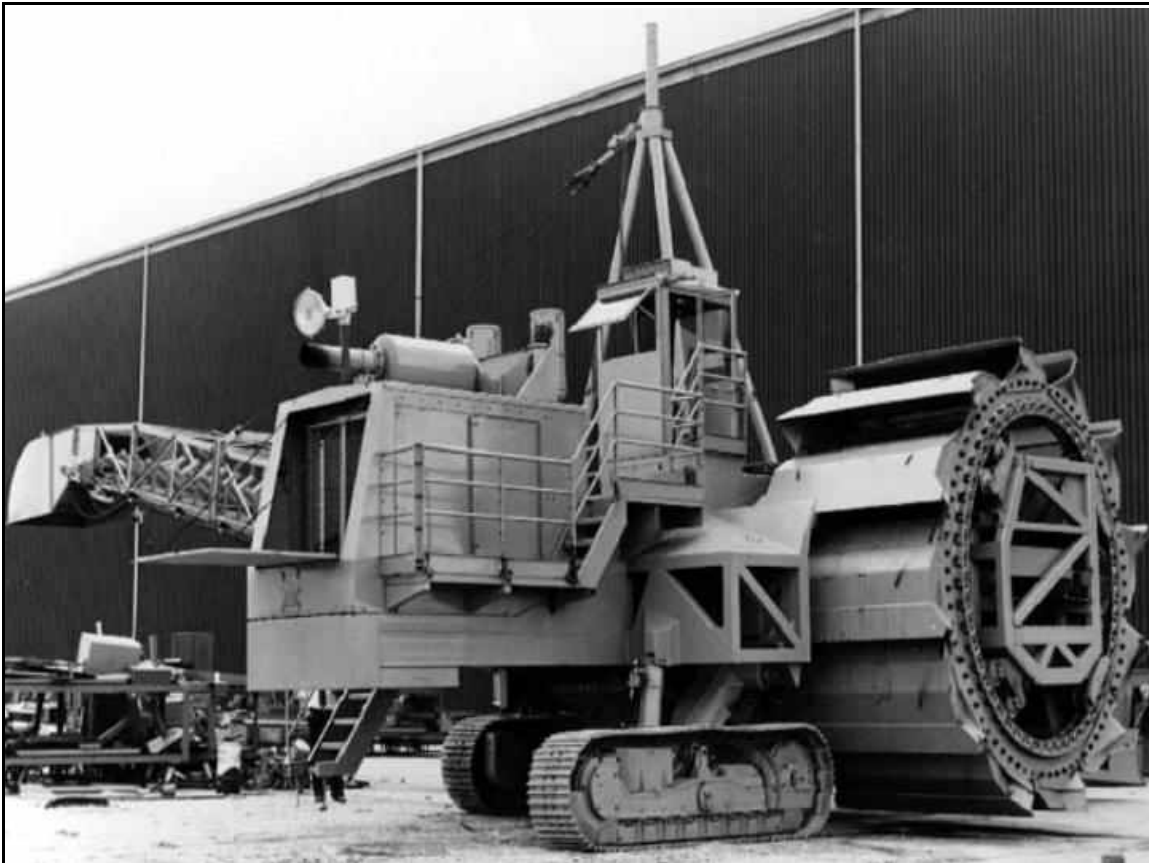
Figure 6. Conventional tracked wheel excavators are used in mining and materials handling situations. The machine could be adapted with wider tacks and other features to operate in shallow water in Upper Peoria Lake. The excavator discharges to a conveyor belt.
