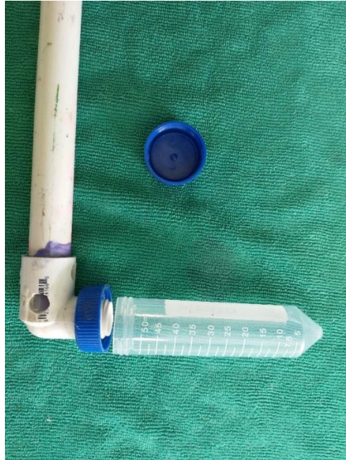
Figure 5. A custom-built sampling device for drainage water collection
