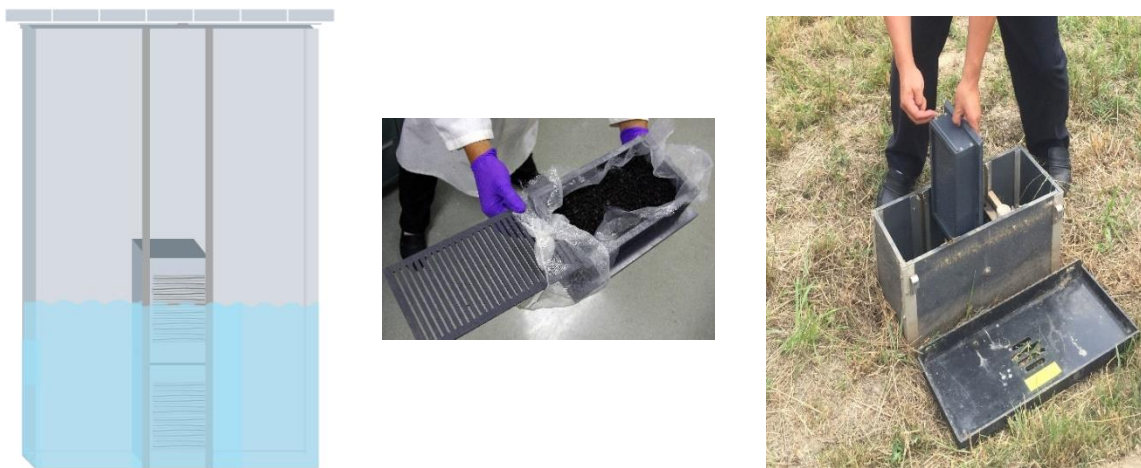
Figure 2. Biochar-sorption-channel with refillable biochar sorption filters
